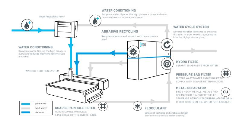
The modules of the OneClean system can, depending on the customer requirements, be combined and added individually. The modern process visualisation system with touch display informs about all processes at a glance.
